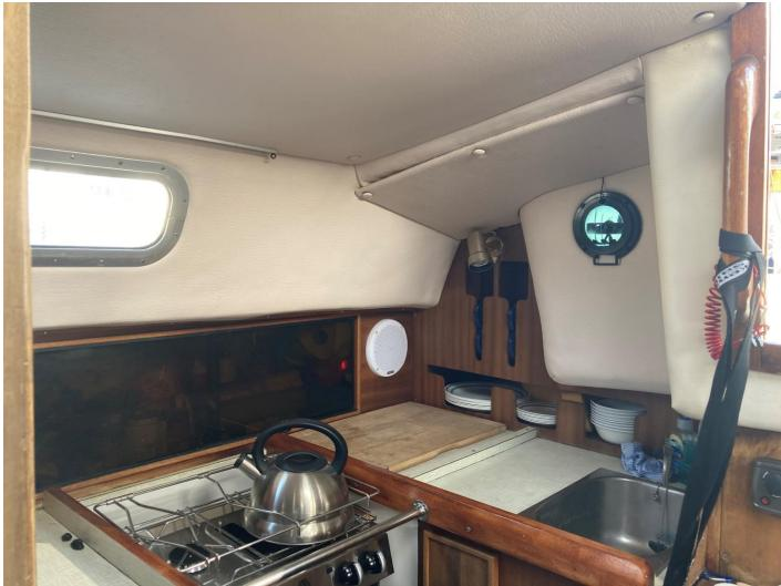
For headlining panels and the trim round the forward hatch, these are best if screwed in place. These buttons and studs are used to hide the screws.
