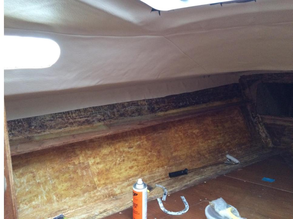
The anchor locker bulkhead has been covered and the port shelf. Wrapping the shelf is made easier as the front edge is straight. Again, remove the foam from the vinyl lip fixed to the hull.
