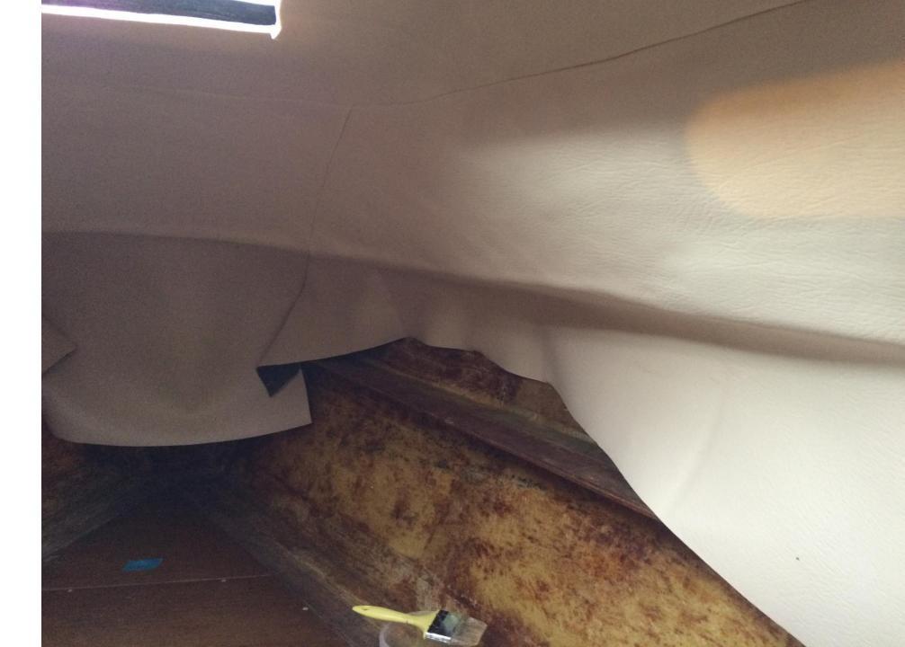
Now fix a strip down the hull about 4" wide. It is best to remove the foam from this strip.
