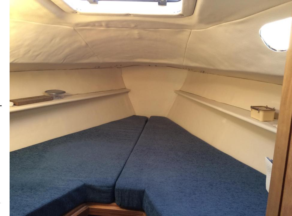
The port shelf has been relacquered before being refitted. Notice how neat the cut at the top of the hull lining is. A snap off knife and a steel ruler were used to just cut the vinyl, not the foam. Once cut through, it was glued in place.
