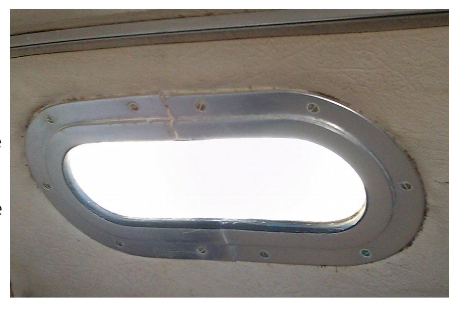
This is what you are left with, it looks a mess. You do not need to remove all the old adhesive, just make sure there is no old foam left. The upper port hull side still has old foam. Scrap it off and leave no lumps of old adhesive.
