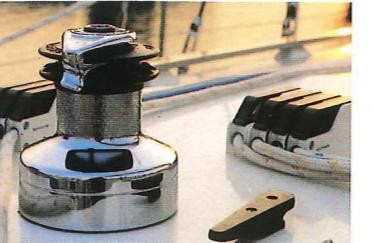
There's a sense of purpose about thoughtful touches like the standard headsail furling drum being placed below the deck, and all the lines being led to self-tailing winches in the cockpit for easy handling in both sloop and cutter versions.
