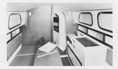
Each layout has two full length berths in the separate forecabin and two full length berths in the aft cabin. In the 'Type A' layout the table lowers to make a double berth; in the 'Type B' layout a double berth conversion for the L-shaped dinette is available as an option. There is an enclosed head to port and opposite is a hanging space. All cabins are lined with an easily cleaned vinyl headliner with foam backing, to minimise condensation.
