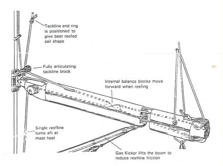
Single line reefing is suitable for conventional and fully battened mainsials. The addition of
