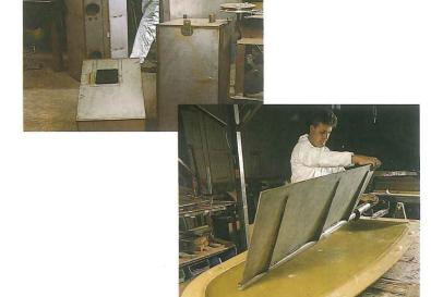
Every Westerly rudder has a stainless steel stock positioned by hand inside a two-part glassfibre blade shell, which is then filled with resin mix and laminated together under pressure. Our way ensures the finished article is as strong as possible, using an alliance of the right materials and the best techniques.
