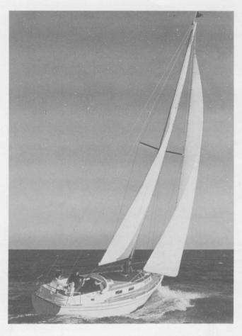
Westerly 35, designed by Laurent Giles & Partners, is a fin keel, aft cockpit sailing cruiser based on the well proved Conway hull. She is designed and built for passage-making and offers a high degree of comfort for the cruising family. Wheel steering and sloop rig are standard and she is supplied with a 42 hp diesel. Ketch rig is available at an extra cost.
