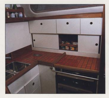
Galley situated to port, aft of the saloon is well-appointed, with useful features such as twin sinks supplied from a stainless steel tank and extra Westerly touches such as tasteful ceramic tiling and a pressurised hot and cold water system. There is plenty of cupboard space and the entire galley area is easy to clean.
