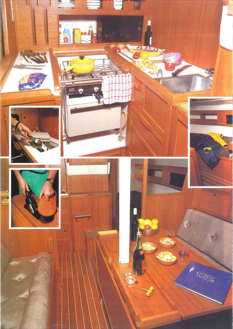
**Galley** The galley is to starboard and is comprehensively equipped with stainless steel sink, hot and cold pressure water supply, large ice box, work top and a gimballed two burner cooker complete with oven and grill.
