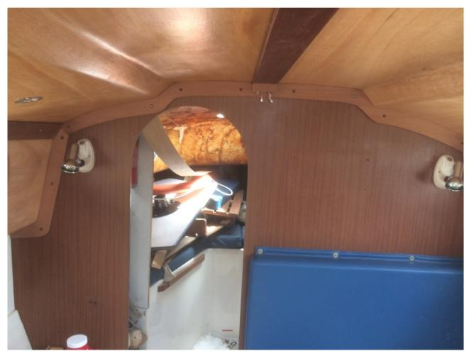
All in all headroom is only reduced by around 12mm which is still standing headroom in my case (5'101/2) and it's a job that unless the boat sinks (and then it doesn't matter) will never need doing again. If required it could be changed with a coat of paint.
