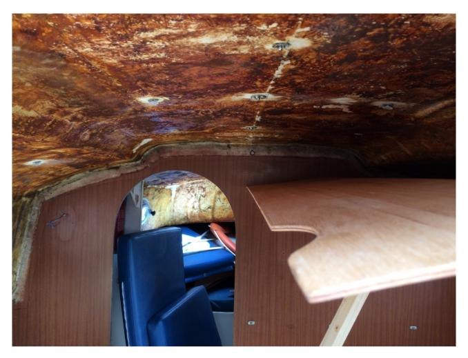
The outer edge of the ply is dropped into a groove in the covering board which is carved from Utile. This holds the top edge of the side panel and the outer edge of the ceiling panel.
