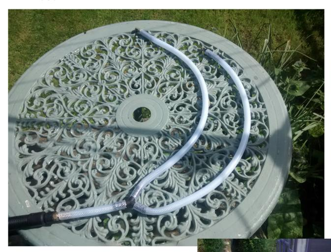
Three short pieces of pipe joined with a Y piece to the steamer outlet pipe. The longer two pipes having holes one inch apart all the way along and a bung in the end to force the steam out of the holes.
