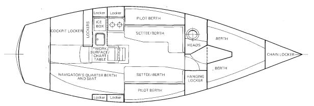
\*The Chart Table and Hinged Work Surface are below the Bridge Deck and on top of the Engine Box.
