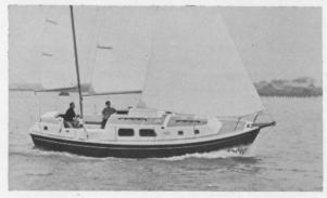
The hull of Renown is identical to that of Longbow. Her accommodation provides three separate cabins and a centre cockpit which is more spacious than is normal for a boat of this length. Like Longbow she provides enjoyable extended cruising and has proved to be a well balanced, easily driven boat. Renown is available as a sloop or a ketch.
