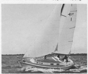
This shoal draft off-shore sailing cruiser combines the advantages of twin keels with the ability to make ocean passages. The main features are the 12' 5" (3.78 m) main cabin and the large aft cockpit. There is a generous amount of space for the chart and galley areas and plenty of lockers for personal and sailing gear. There is a choice of ketch or sloop rig and a powerful diesel auxiliary is fitted as standard.
