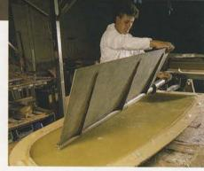
Every Westerly rudder has a stainless steel stock positioned by hand inside a two-part glassfibre blade shell, which is then filled with resin mix and laminated together under pressure. Our way ensures the finished article is as strong as possible, using an alliance of the right materials and the best techniques.
