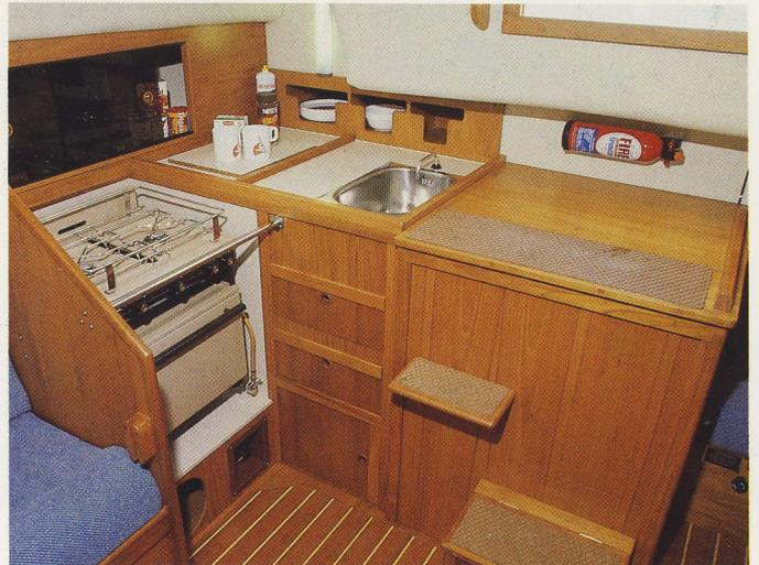
There is a large stainless steel sink supplied from a 30 gallon stainless steel fresh water tank.
