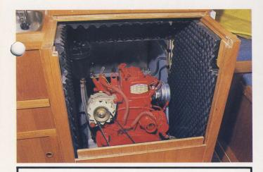
**Engine** Power for the Fulmar comes from the very reliable and smooth running 18hp 2-cylinder diesel engine, which gives a hull speed in excess of 6 knots plus power to spare. The 20-gallon fuel tank gives a cruising range of over 200 miles.
