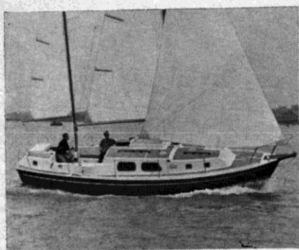
RENOWN KETCH (including 25hp diesel engine) LOA LWL Beam Draught Sail Weight 32ft 6in 25ft 9ft 6in 4ft 6in 440sq ft 10083 lb 9.9m 7.6m 2.9m 1.38m 41.0sq m 4923kg Sloop rig also available
