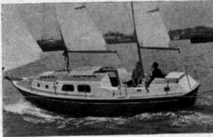
PENTLAND KETCH (including 25hp diesel engine) LOA LWL Beam Draught Sail Weight 32ft 6in 25ft 9ft 6in 3ft 7in 440sq ft 10163 lb 9.9m 7.6m 2.9m 1.1m 41.0sq m 4960kg Sloop rig also available
