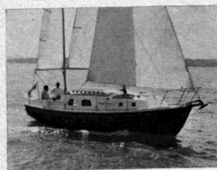
BERWICK KETCH (including 25hp diesel engine) LOA LWL Beam Draught Sail Weight 32ft 6in 25ft 9ft 6in 3ft 7in 440sq ft 9863 lb 9.9m 7.6m 2.9m 1.1m 40.9sq m 4450kg LOA includes bowsprit. Sloop rig also available
