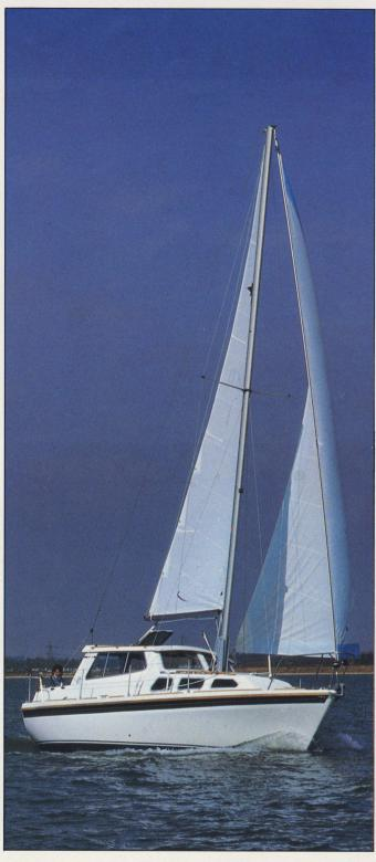
The rig is developed from the Konsort design, offers a single spreader masthead rig and deck stepped mast with a good sail area for real sailing performance. It is designed to be easy to handle, even when sailing short-handed.
