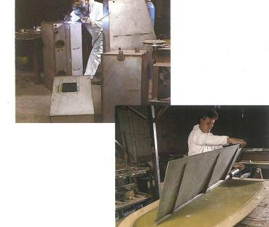
Every Westerly rudder has a stainless steel stock positioned by hand inside a two-part glassfibre blade shell, which is then filled with resin mix and laminated together under pressure. Our way ensures the finished article is as strong as possible, using an alliance of the right materials and the best techniques.
