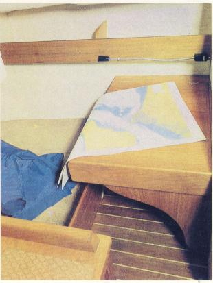
**Quarter berth** – to port with stowage bins under. All the internal hull surfaces are fully lined against condensation with the deck head areas with removable ply panels, allowing easy access for additional deck fittings, wiring runs etc.
