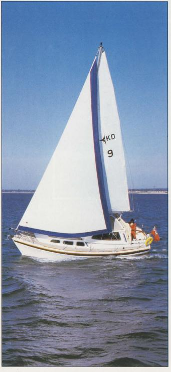
The rig is developed from the Konsort design, offers a single spreader masthead rig and deck stepped mast with a good sail area for real sailing performance. It is designed to be easy to handle, even when sailing short-handed.
